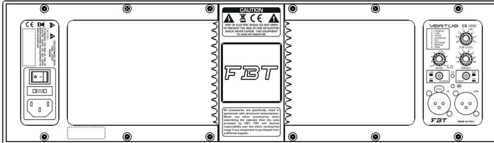
The subwoofer display a high-efficiency Class D power amplifier module with switching power supply enclosed in a die-cast aluminium chassis. This permits to protect the electronics against dust, avoid any air loss through the controls which would cause annoying noises, maximize heat loss by using the woofer ventilation instead of a cooling fan.
